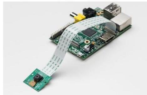
Pic 5: Raspberry pi 2 kit with Pi camera
