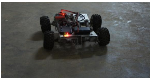
Pic 13: Field test of UGV with Raspberry kit
